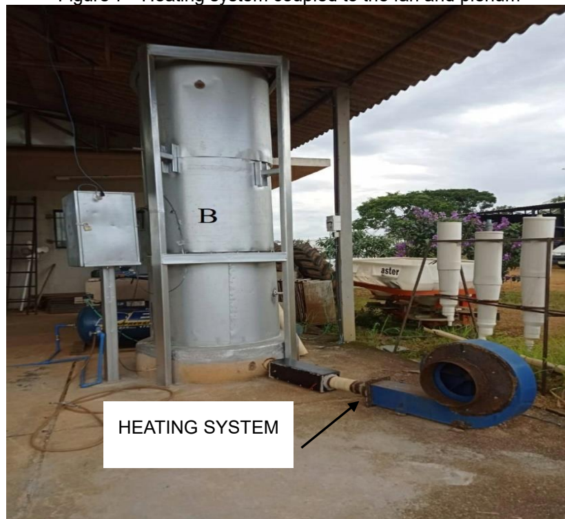
Figure 7 - Heating system coupled to the fan and plenum
