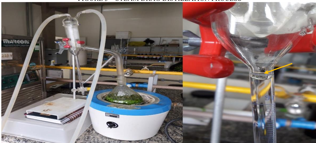
FIGURE 3 – STEAM DRAG DISTILLATION PROCESS
