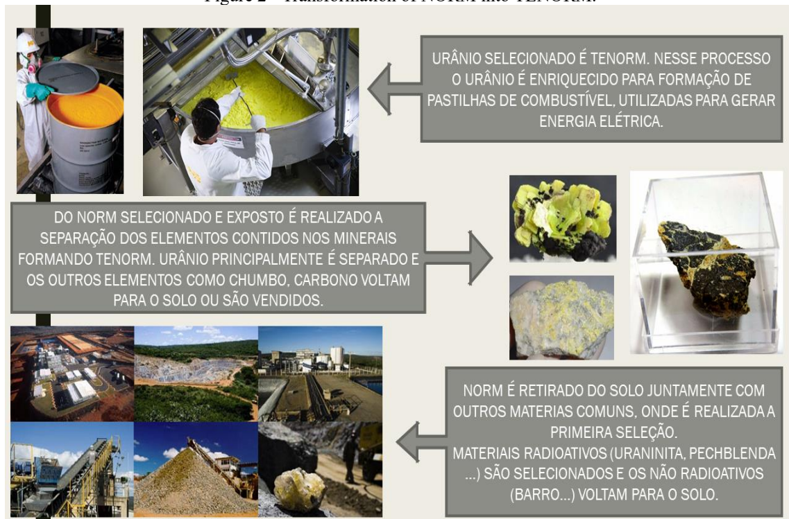
Figure 2 - Transformation of NORM into TENORM.
