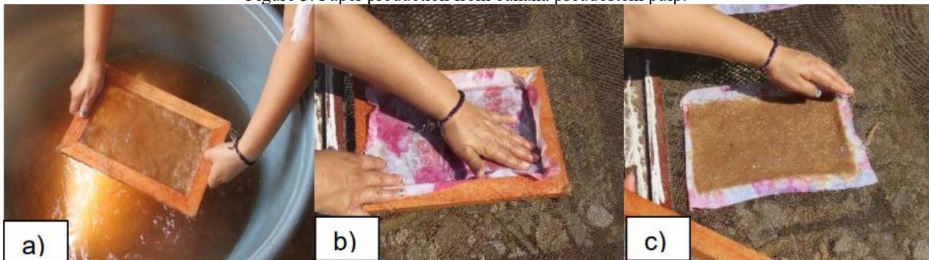
Figure 3. Paper production from banana pseudostem pulp.
