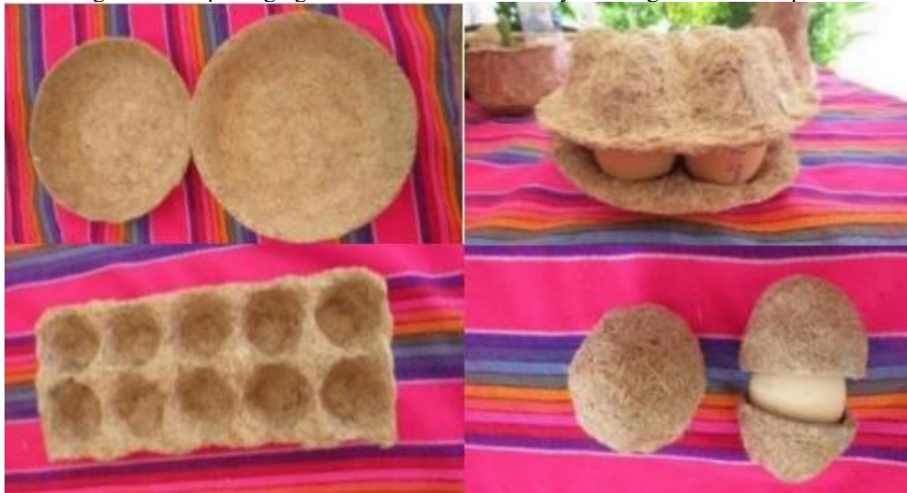
Figure 8. Bio packaging and containers obtained by molding banana fiber paste.
