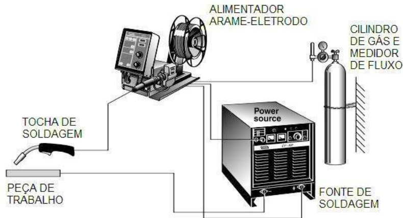
Figure 9: GMAW Soldering Circuit
