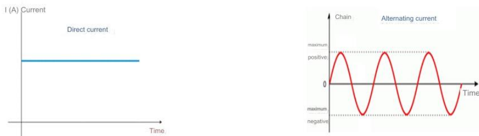
Figure 3 - Graphs of DC and AC currents as a function of time.
