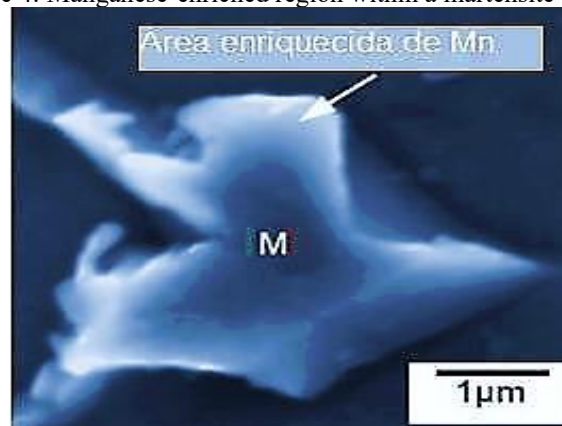
Figure 4: Manganese-enriched region within a martensite particle
