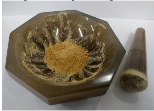
Figure 2: Wax being crushed in agate mortar
