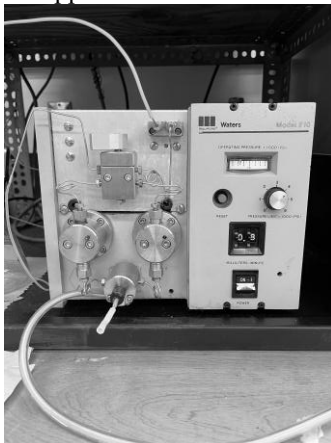
Figure 2 – Detail of injection of eluent and polymer solutions at Size exclusion chromatography (SEC) equipment and their apparatus for molecular mass determination.
